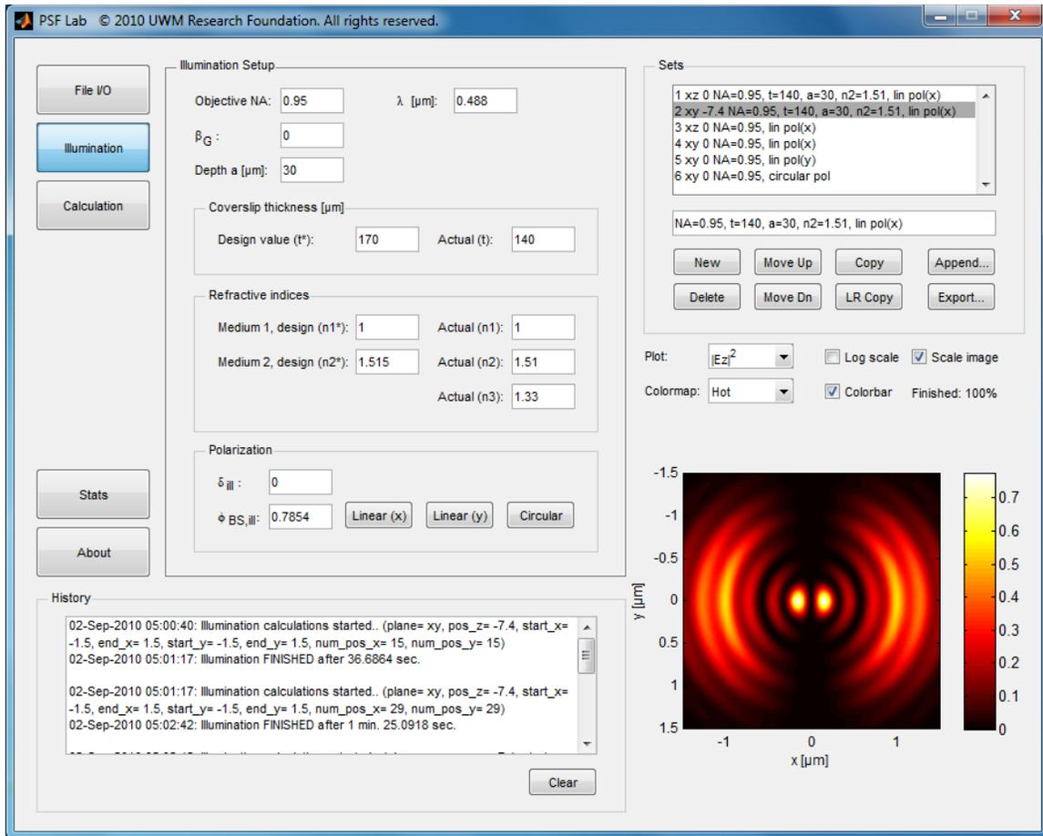
**Coverslip thickness [ $\mu\text{m}$ ]:** design value,  $t^*$ , and actual (= real) thickness,  $t$ , of the coverslip that supports the sample medium. Units:  $\mu\text{m}$ .
