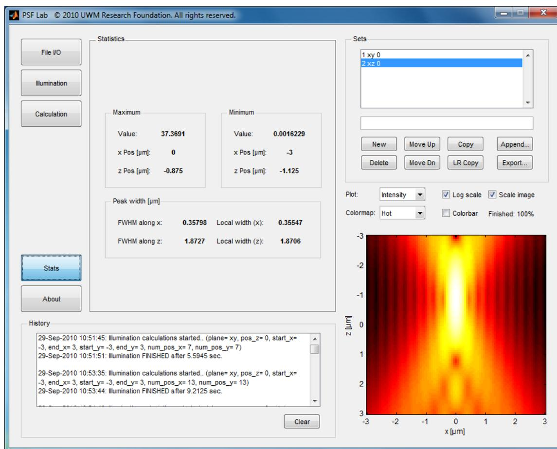
The extension of the focal spot in the  $z$  direction is about  $1.9 \mu\text{m}$ , more than five times larger than its lateral extension (along  $x$ ) of about  $0.36 \mu\text{m}$ . Note that the value for the width along  $x$  is somewhat smaller than the  $0.38 \mu\text{m}$  that we had calculated for the  $xy$  image. At closer inspection this is not surprising, however, since the  $xy$  calculation was carried out at  $z = 0$ , which is  $0.875 \mu\text{m}$  away from the true focal spot.
